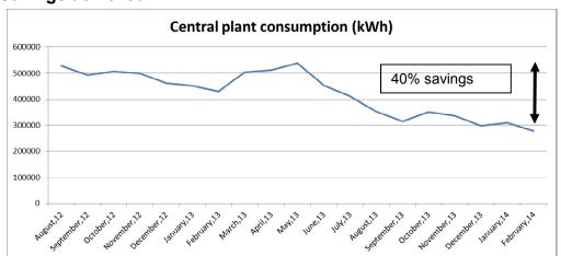
Chiller system efficiency improved from 1.0 to 0.65 kW/RT
